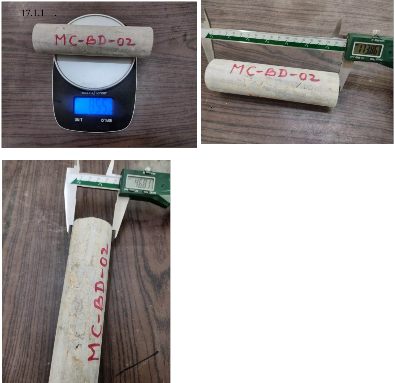
Figure 10: Photographs showing procedure of determination of length, diameter and weight of sample number MC-BD-02 for bulk density calculation
