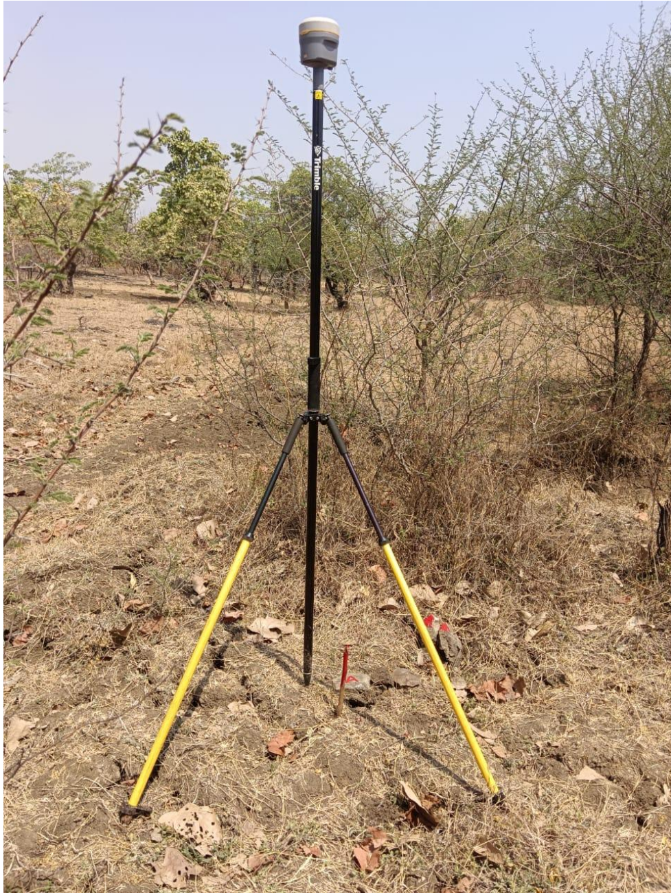
Figure 7: Fixing of block boundary corner point “A” with the help of DGPS
